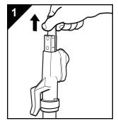
Before assembling appliance, remove two screws from connector assembly. Remove cardboard insert by pulling upward.
